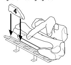
Figure 46 - Installing Log No. 4
